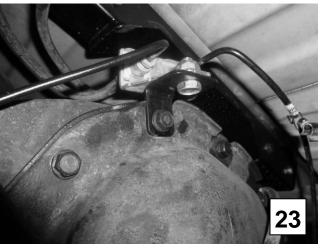
4u) Reinstall gas tank and shield. Make sure all hoses and clips are reattached.
