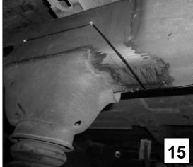
**4e)** Connect the lines marked for the inner and outer templates across the bottom of the frame.(**Photo 15**)
